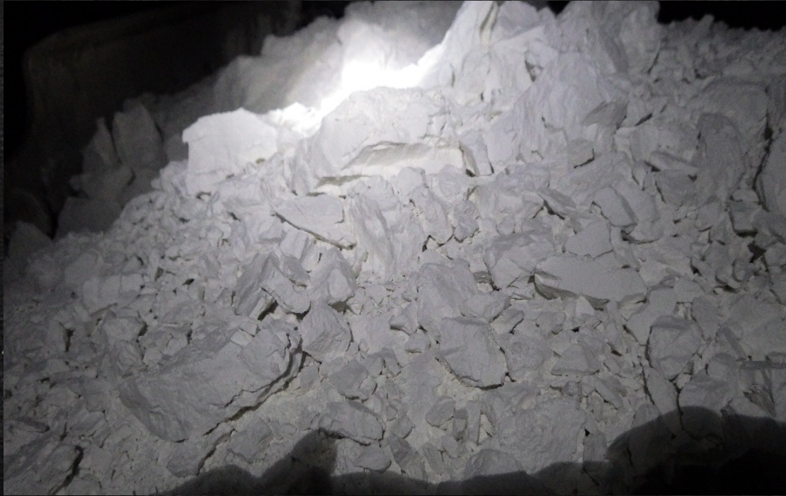
Un-treated rock dust in scoop applied at Stockton Mine
