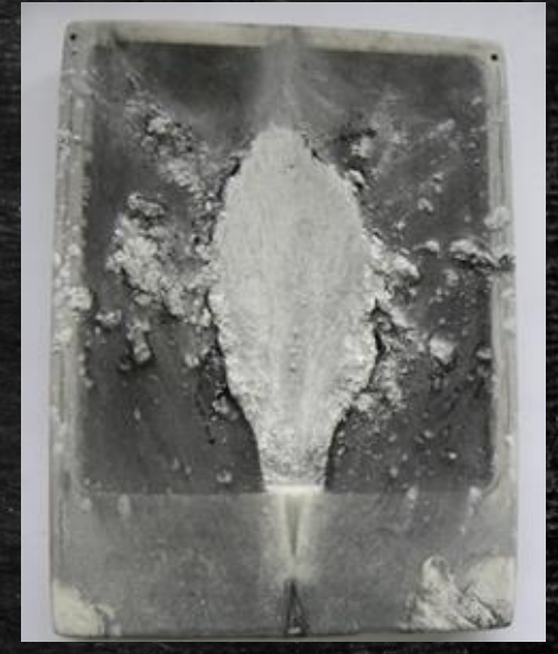
Coal dust on top of treated rock dust (Exposed to water and dried)
